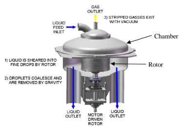
Figure 1 - The GasTran Unit as Set Up for Vacuum Deaeration
