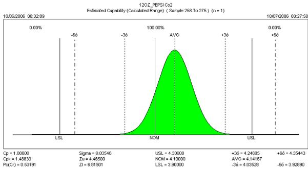
**Figure 6 – Carbonation Levels after Installation**
