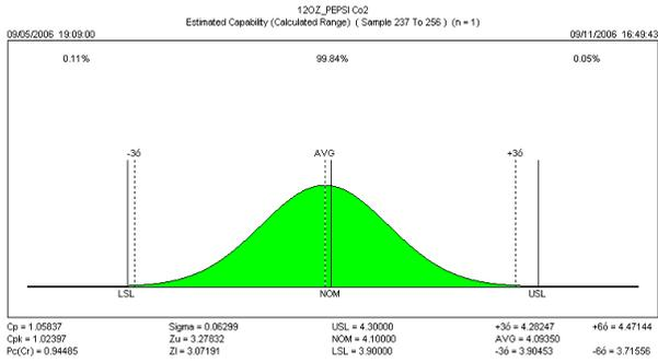
**Figure 5 – Carbonation Levels Prior to Installation**
