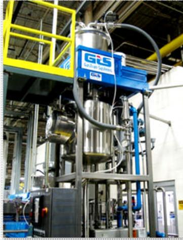
**Figure 4 - GasTran Deaeration System Installed in Austin, IN**
